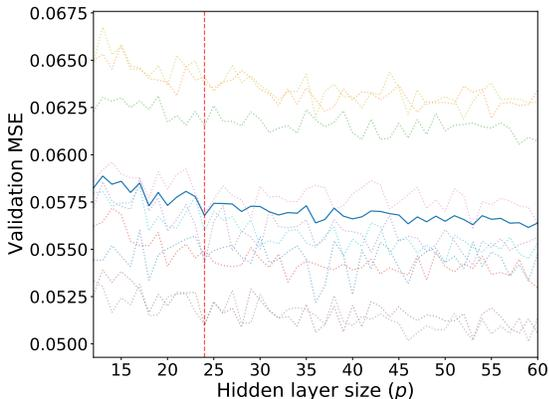
Fig. 10. Mean validation MSE (solid blue line) vs. hidden layer size ( $p$ ) across 10 repeated validation runs (pale dotted lines). Improvements are insignificant past  $p = 24$  (vertical dashed line).
