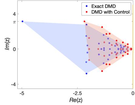
Fig. 8. Plot of the distribution of logarithm of eigenvalues of  $A$  derived from Exact DMD and DMD with Control. The blue markers and light blue region visually represent the dynamics when GRYD is viewed as endogenous for the system. The red markers and red region show the dynamics of the same participants when GRYD is hypothetically not in action.
