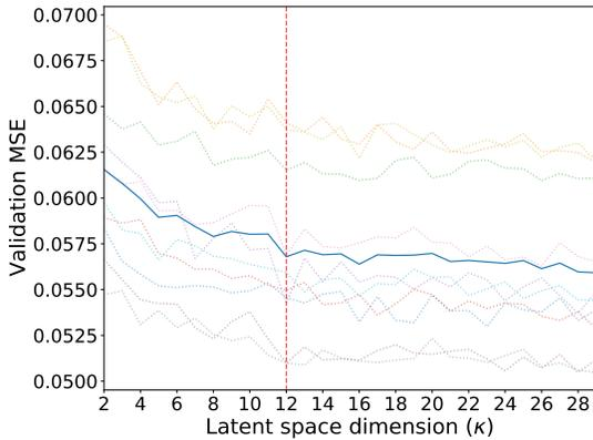
Fig. 9. Mean validation MSE (solid blue line) vs. latent space dimension ( $\kappa$ ) across 10 repeated validation runs (pale dotted lines). Improvements are insignificant past  $\kappa = 12$  (vertical dashed line).
